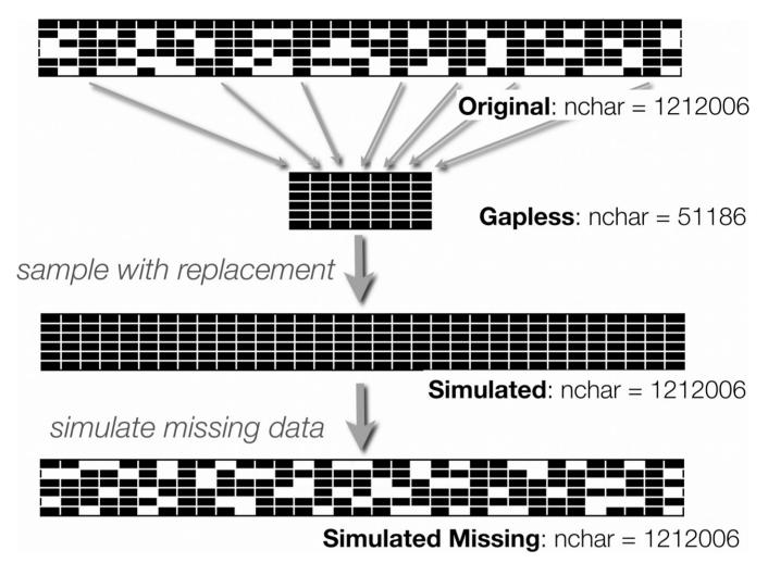
FIG. 1. Simulation of data sets to test the effect of missing data. In the original alignment, missing data is distributed unevenly among the species. In the final simulated alignment, missing sites are distributed randomly among the species.
