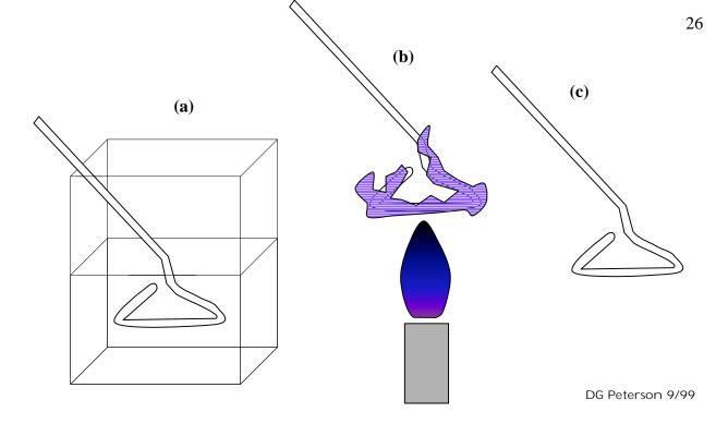
**FIGURE 5.1** - Alcohol sterilization of a glass plating rod. (a) The "hanger-shaped" end of the rod is inserted into a container in which 70% ethanol has been placed. (b) The alcohol drenched rod is ignited by quickly passing it into the flame of a Bunsen burner or alcohol lamp. (c) The alcohol on the end of the rod is allowed to burn away. The rod is allowed to cool for several minutes before further use.
