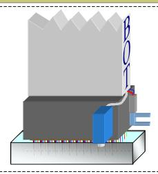
(d) Once the picking cycle is initiated, the OBot's first order of business is to sterilize the picking pins. In brief, the robotic arm places the bottom of the picking head (i.e., the pins) into the ethanol wash bath. The arm makes a series of short, jerky movements effectively moving the pins back and forth through the bath. Groups of clustered bristles lining the bottom of the enhance bath the cleaning process.
