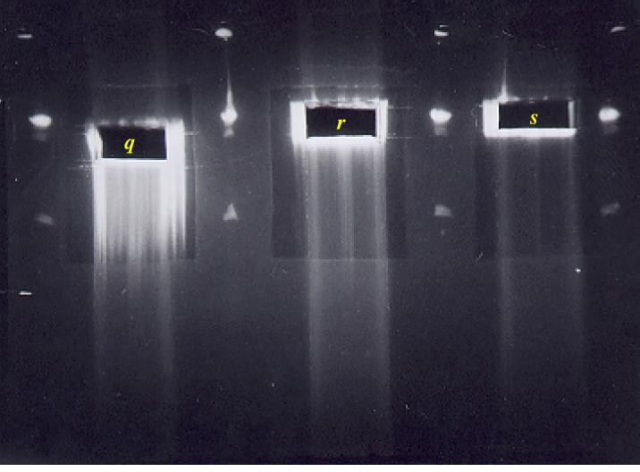
**FIGURE 12.2** - Partially-reconstructed gel after a second size selection. This gel shows DNA from *Saccharum officinarum* (sugarcane). Blocks q, r, and s containing unstained DNA between 125 and 350 kb have been removed from the gel as described in FIGURE 12.1. The spaces where blocks q, r, and s were located have been labeled.
