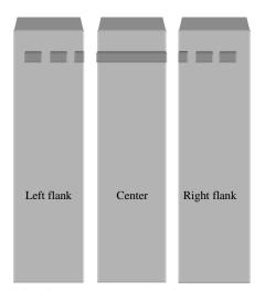
(**b**) After electrophoresis, divide the gel into three pieces as shown. The two flanking pieces should each contain a small part of the slot-well as well as a DNA ladder. Stain the flanking pieces with ethidium bromide. Do not stain the center piece (the gel piece containing most of the vector DNA).
