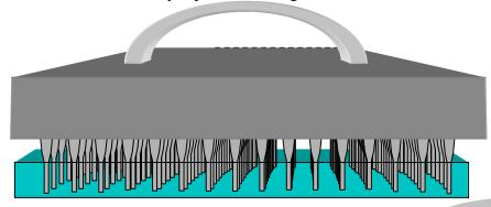
(a) The stainless-steel replicator is placed in a 70% ethanol bath. The replicator is gently moved back and forth through the ethanol to ensure that the pins are thoroughly cleaned. The replicator is removed from the ethanol bath, and the residual ethanol on the pins is
