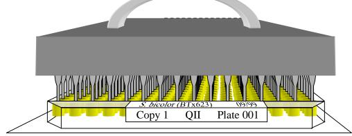
(c) The replicator is inserted into the wells of a plate containing sterile freezing medium. This newly-inoculated plate should be labeled "Copy 1, Plate 001", and the replicator should be inserted into the plate in exactly the same orientation as it was inserted into the master plate. The lid of Copy 1, Plate 1 is replaced, and the plate is set aside.
