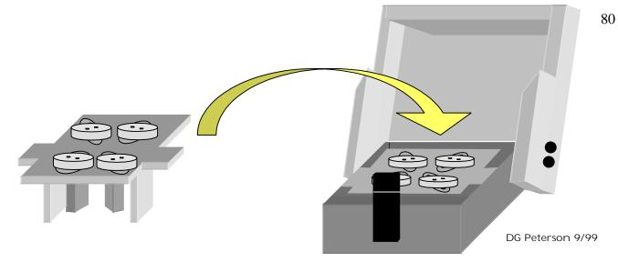
**FIGURE A.3** - Loading the chamber safe. Four cuvettes loaded with transformation mixture are placed into the cuvette holder. The filled holder is then gently inserted into the ice-filled chamber safe.
